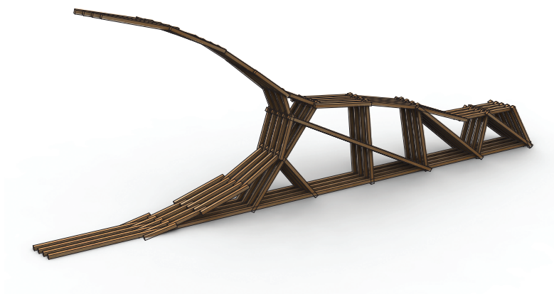
1:1:10 Final assembly of one set of components, which are screwed to subsequent sections.
